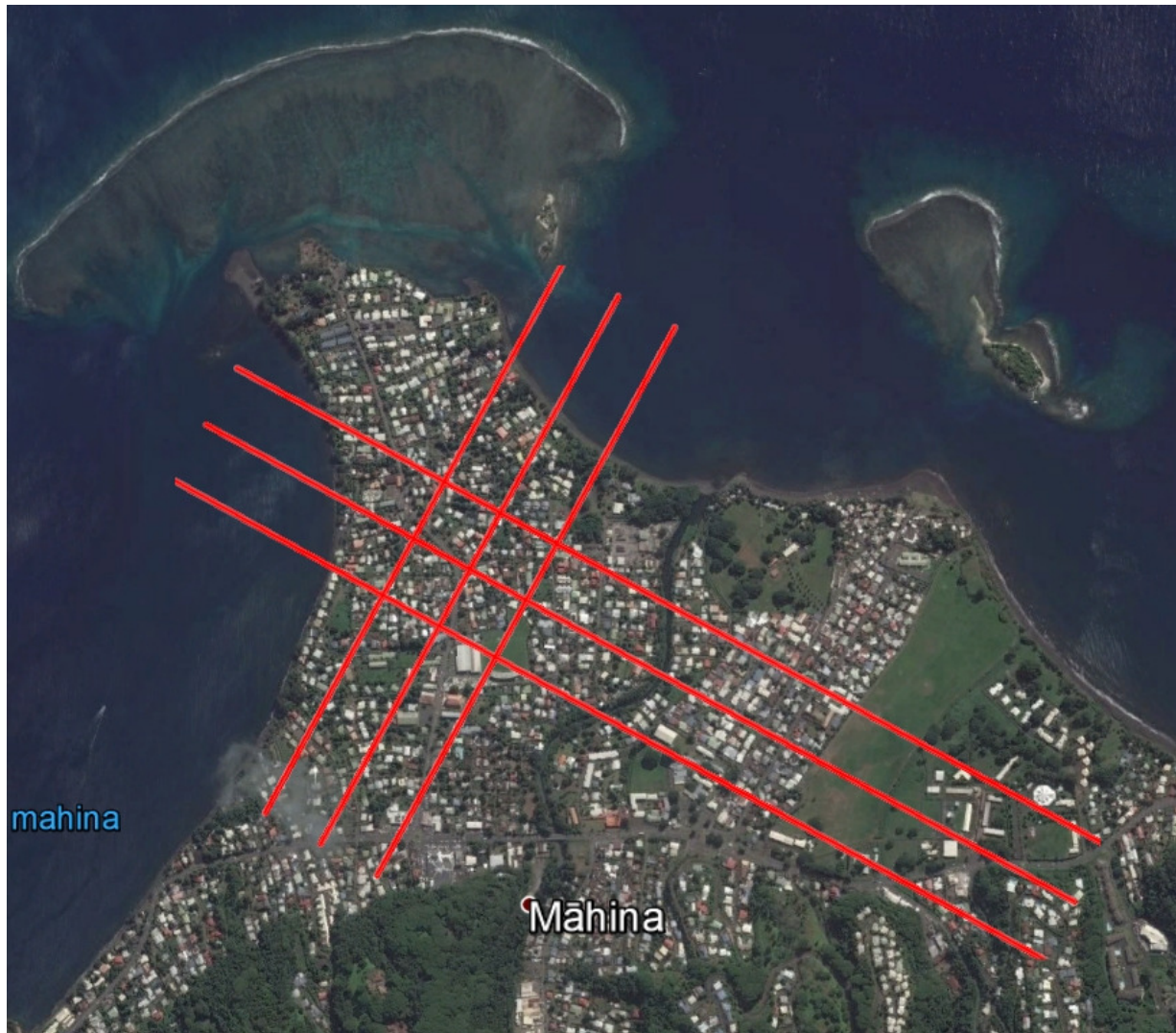
Figure 4: RIEGL VQ-820-G calibration flight plan
